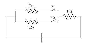
**Q.11** When switch  $S_1$  is closed and  $S_2$  is open, the circuit resistance is  $R_3$ . When switch  $S_1$  is open and  $S_2$  is closed, it is  $R_4$ . When both switches are closed, it is  $R_5$ . It is given that  $R_3 : R_4$  is 8 : 5 and  $R_3 : R_5$  is 2 : 1. Find the value of  $R_1$  in ohms. (The battery is ideal.)
